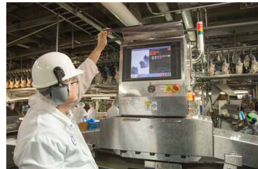
Plant manager David Rackley monitors one of nine Anritsu x-ray machines that ensure products contain no foreign matter.
