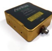
(b) 110 GHz NLTL VNA Frequency Extender
