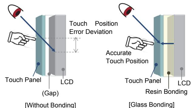
Figure 3 Glass Bonding Effect
