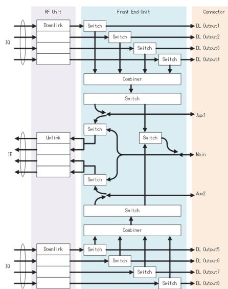
Figure 2 Transceiver Block Diagram
