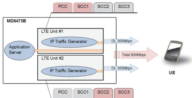
Figure 6 Dual-Unit Configuration
