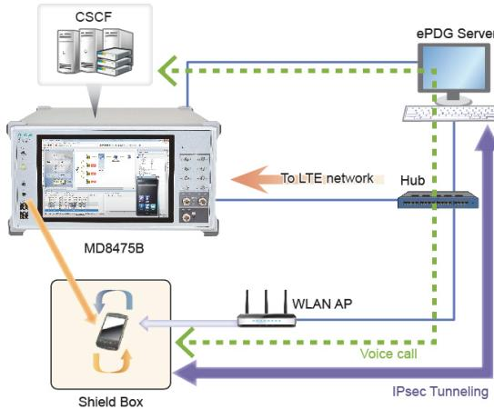
Figure 12 WLAN Calling Test Environment
