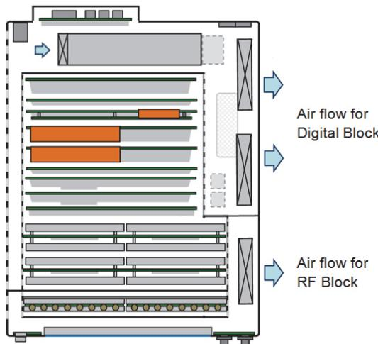
Figure 4 MD8475B Main Unit Internal Layout
