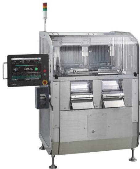
Figure 1 External View of KWS9001AP20 Capsule Checkweigher
