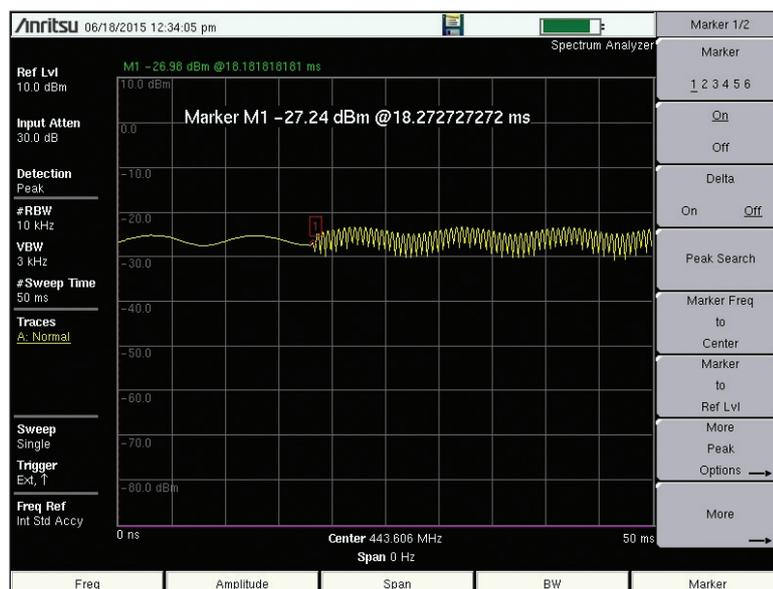
Figure 3. Delay through a Motorola Quantar in NBFM mode. The slower audio waveform before the 2 kHz burst is the 105 Hz PL tone from the repeater.
