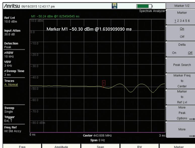
Figure 5. Audio Delay through a Motorola GR1225 analog repeater.
