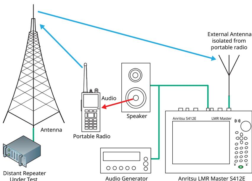
Figure 1. Block Diagram for Audio Delay Measurement.
