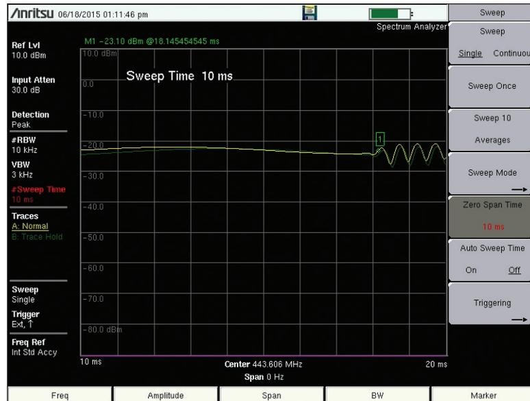
Figure 4. Delay through a Motorola Quantar with 10 MS trigger delay. Note the green trace is a reference and the yellow trace a second measurement with a 40 us audio delay to the speaker.
