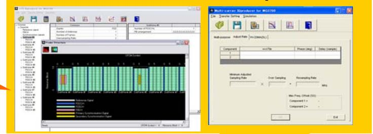
Adjust frequency offset and power level difference on screen
