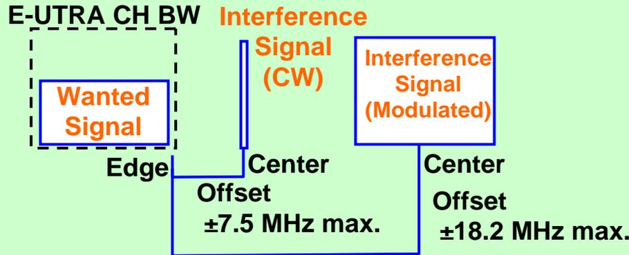
**Interference signal (Modulated/CW)**
