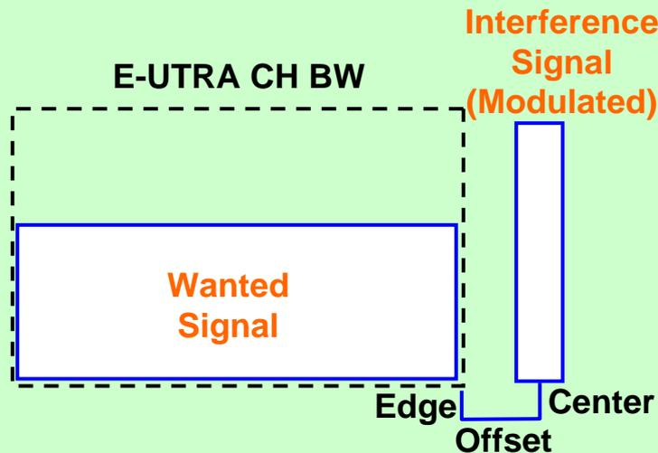
Wanted signal      Interference signal (QPSK)
