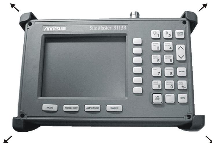
**Figure 4-1.** Removing the Corner Bumpers
