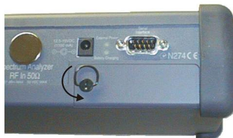
**Figure 3-2.** Rotate the Battery Access Door Handle
