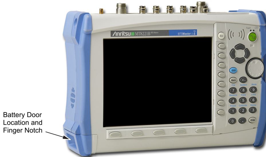
Figure 4-1. Battery Access Door Location and Finger Notch
