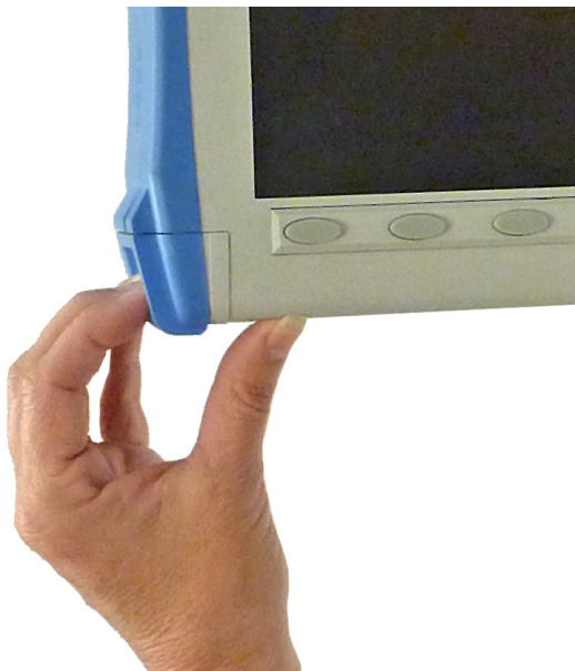
Figure 4-2. Opening the Battery Access Door
