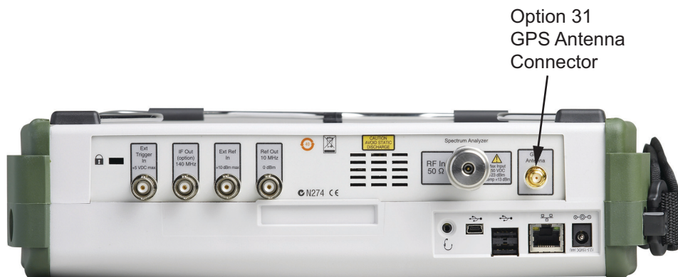
Figure 5-1. Remove Option 31 Lock Nut and Washer
