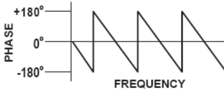
**Figure A-16.** Linear Phase with Frequency Waveform
