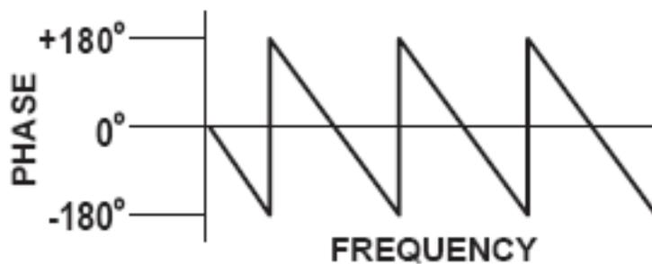
Figure A-16. Linear Phase with Frequency Waveform
