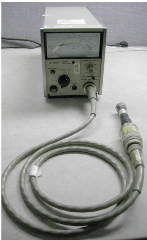
432A Power meter shown connected to the 8478B power sensor.
