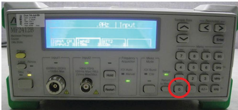
Figure 6-5. MF2412B Input Key
