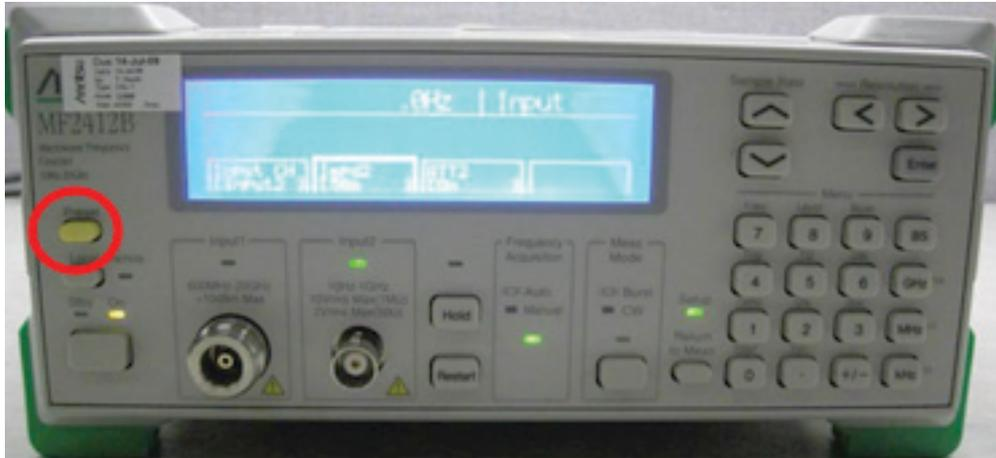
Figure 6-4. MF2412B Preset Key
