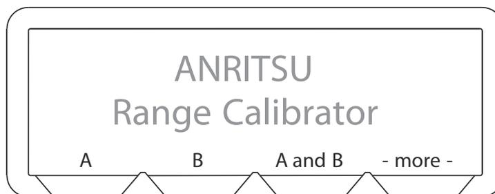
**Figure 4-2.** ML2419A Range Calibrator Top Menu (dual-channel power meter)
