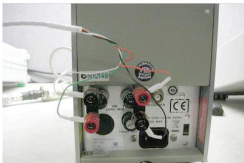
Connection shown to the rear of the 432A power meter.
