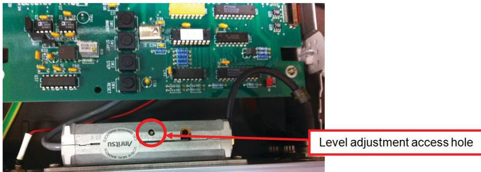
Figure 6-18. Level Adjustment Access
