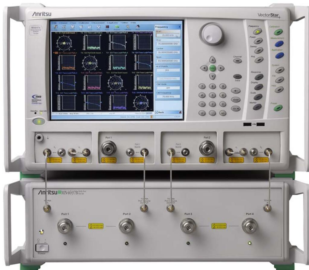
**Figure 1.** MS4647A VNA and MN4697B Test Set System Overview
