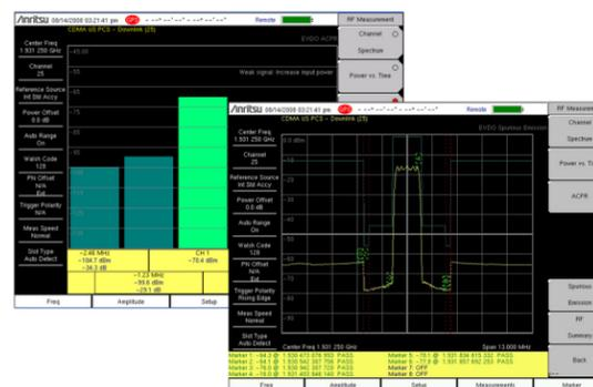
**SEM** is a way to check out-of-channel spurious emissions near the carrier. These spurious emissions both indicate distortion in the signal and can create interference with carriers in the adjacent channels.
