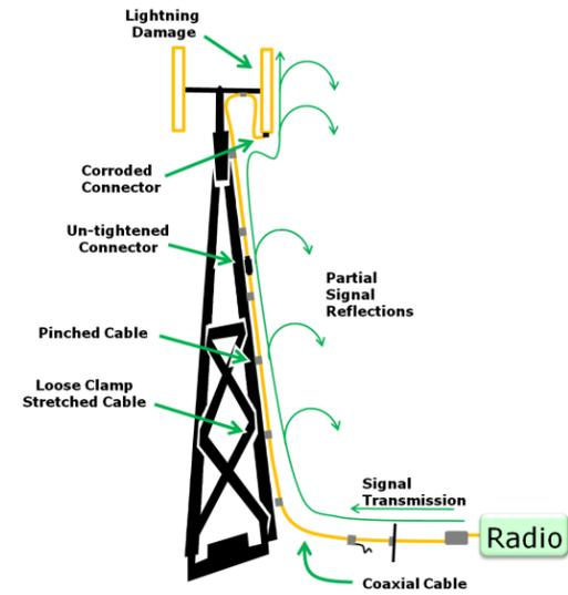
Changes in impedance, in turn, are caused by mismatches, or physical changes in the cable, such as:
