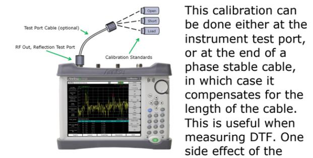
This calibration can be done either at the instrument test port, or at the end of a phase stable cable, in which case it compensates for the length of the cable. This is useful when measuring DTF. One side effect of the high accuracy OSL calibration is that it is dependent on the frequency span of the antenna tester. If the start and stop frequency is changed, the OSL cal will need to be redone.
