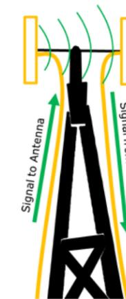
to another. If the leak is strong enough, BTS signal quality can be compromised causing dropped and blocked calls. This sort of problem can affect more than just the radios with poor isolation. Failures mean that the sector is prone to excessive inter-modulation distortion, which lowers signal quality, increases dropped calls, and can cause interference with other radio services.
