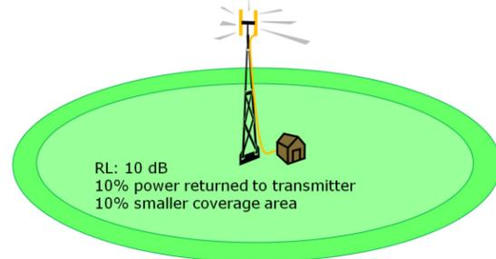
Reduced coverage increases dropped and blocked calls due to weak signal areas and network loading imbalances.
