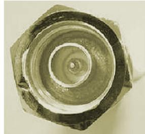
**Common faults** include connector, cable and antenna faults. When looking for faults, it's important to know that most faults are connector related. This includes loose connectors, corroded connectors, and poorly installed connectors. Most remaining faults are cable related. This includes water in the cable, loose weather wrap, pinched cables, poorly installed ground kits, bullet holes, and even nails in the cable! A small portion of the faults are antenna related.
