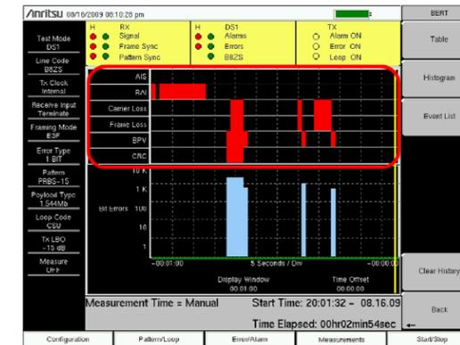
**CRC**, or the Cyclic Redundancy Check numbers, are included in the Extended Super-Frame (ESF) format. If the received CRC and the CRC calculated from the received data do not agree, the received data must be in error.
