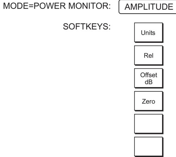
Figure 2-7. Power Monitor Mode Soft Key Labels (Option 5)
