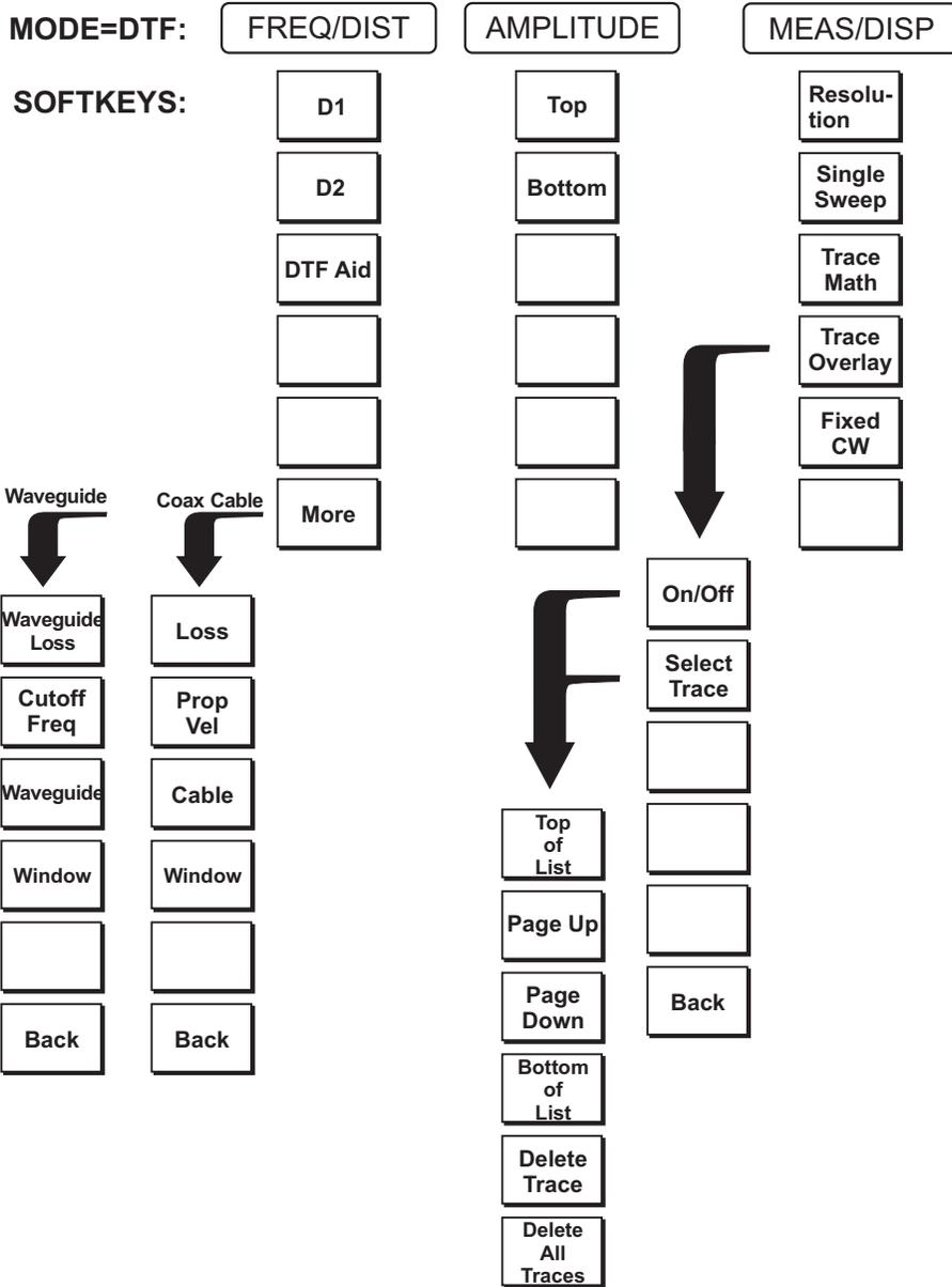
Figure 2-6. Distance to Fault Mode Soft Key Labels
