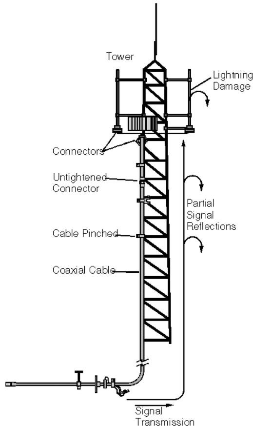
Figure 4-1. A Typical Transmission Feed Line System
