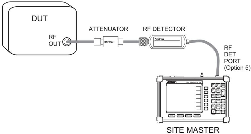
Figure 5-1. Power Monitor Measurement Setup for Absolute Power Measurements
