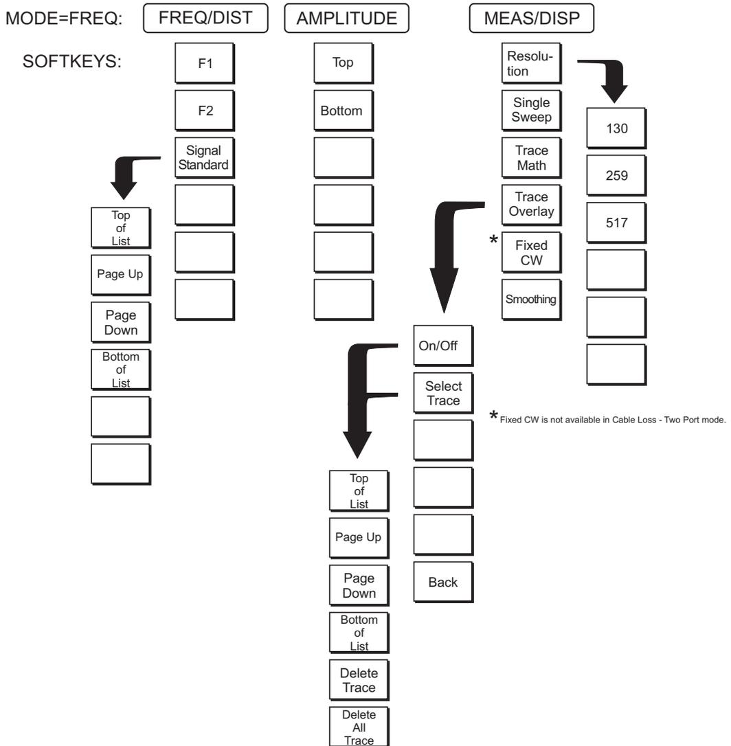
Figure 2-5. Return Loss Mode Soft Key Labels
