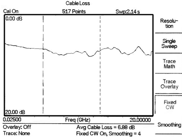
Figure 4-5. Typical Transmission Line Cable Loss Trace with Smoothing Applied
