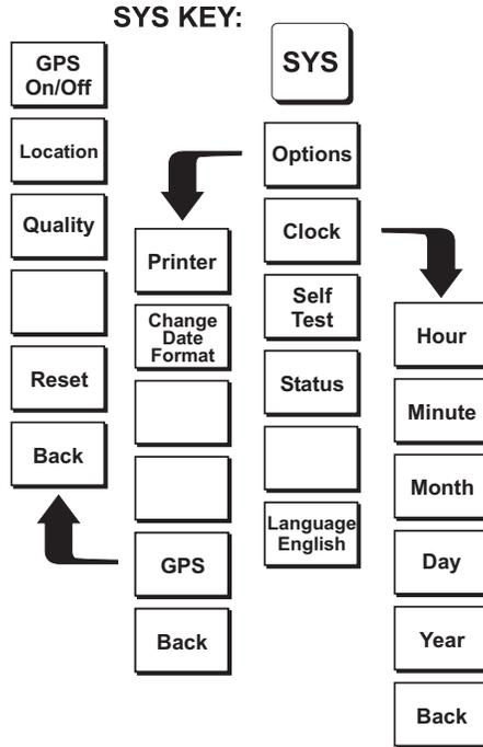
Figure 2-9. SYS Key Menu in Power Monitor Mode
