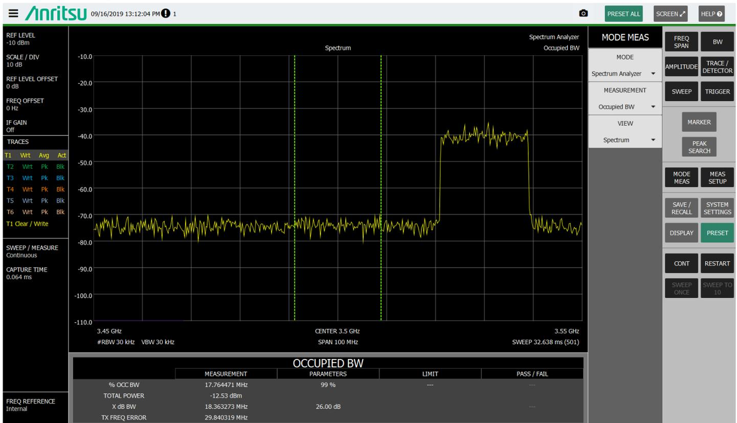
Figure 3: V2019.9.1 GUI example of Occupied Bandwidth measurement, notice that the vertical bars automatically track the signal of interest which is no longer required to be centered in frequency.
