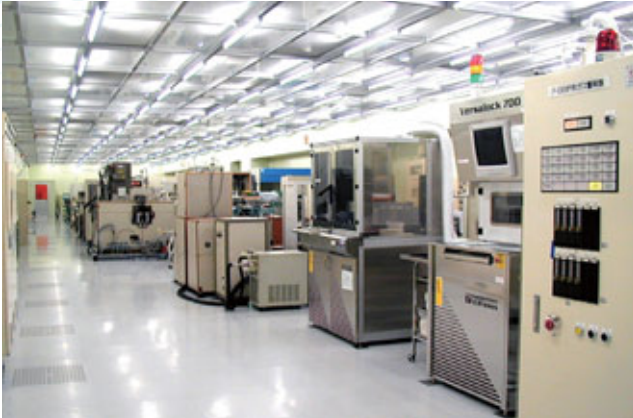
Clean room for MMIC 1 research and development Note 1: Microwave Monolithic Integrated Circuit
