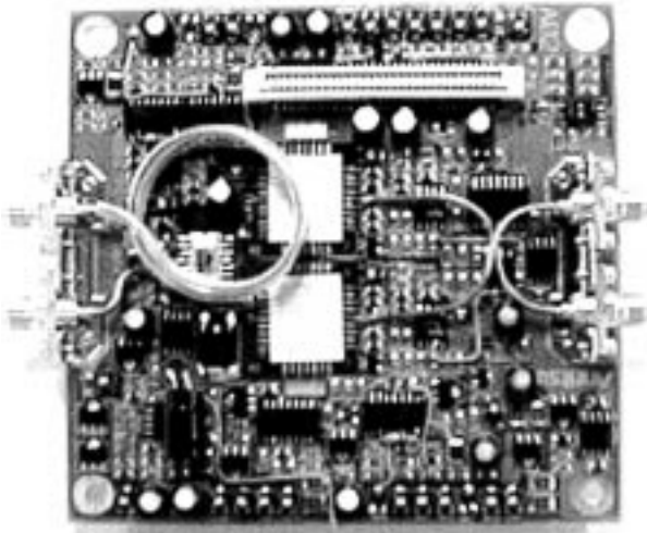
図4 Hybrid ICとバイアス回路 External view of hybrid IC and Bias circuit
