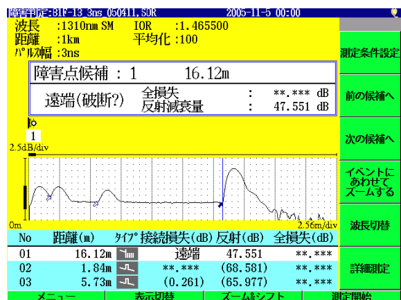
図7 障害判定結果画面 Fault location mode screen
