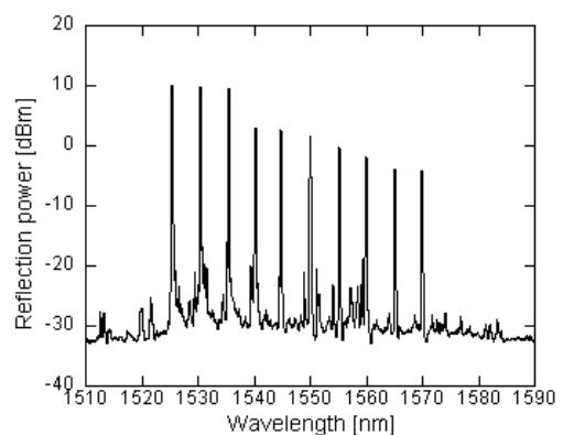
Figure 12 Reflection spectrum of FBG sensors
