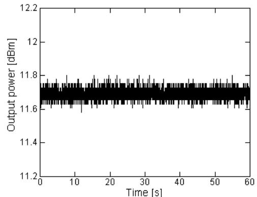
Figure 6 (b) Output power fluctuation for single-mode WSLS at 1550 nm
