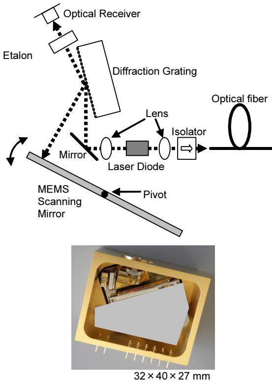
Figure 1 Schematic diagram and overview of single-mode wavelength swept light source (WSLS).
