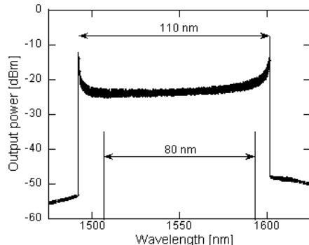
Figure 4 Spectrum of single-mode WSLS
