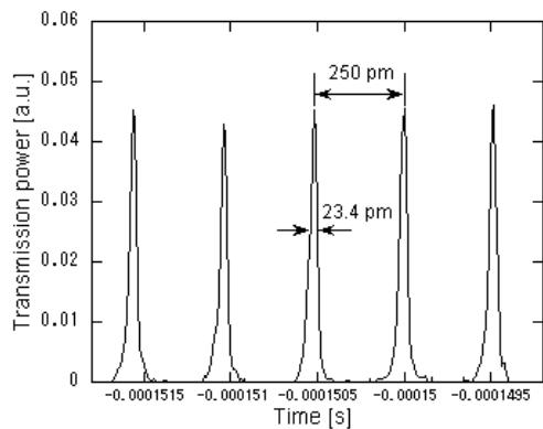
Figure 8 Transmission profile of Fabry-Perot interferometer
