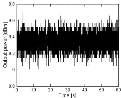
Figure 6 (a) Output power fluctuation for multimode WSLS at 1570 nm
