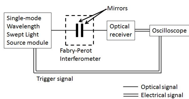
Figure 7 Spectrum width measurement setup
