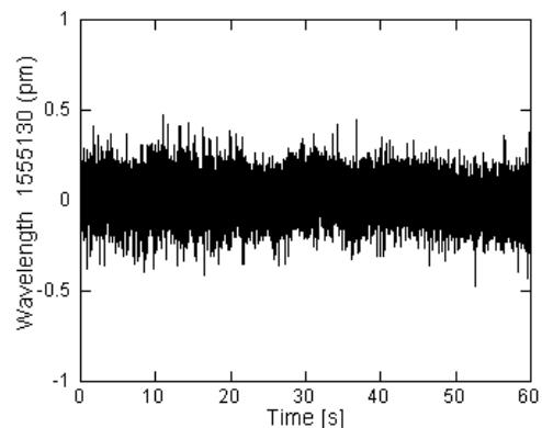
Figure 14 Wavelength fluctuation of center wavelength for FBG sensor at 1555 nm
