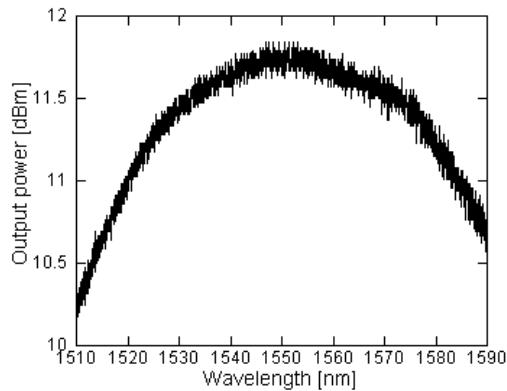
Figure 5 Wavelength dependence of optical output power for single-mode WSLS
