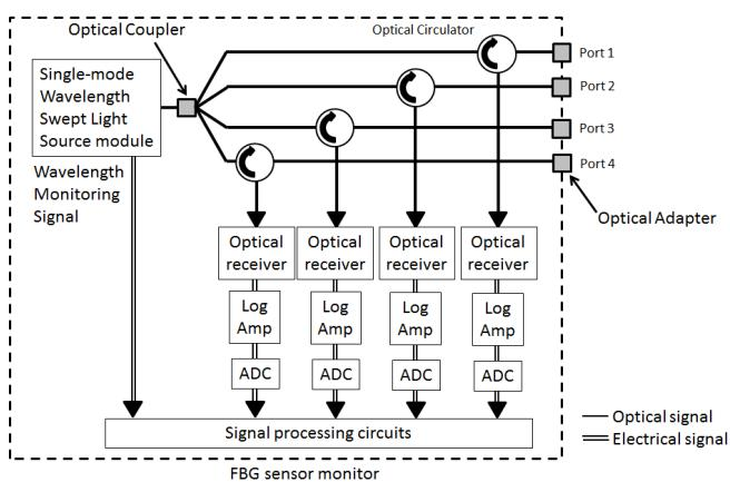
Figure 10 AR4041A FBG Sensor Monitor block diagram
