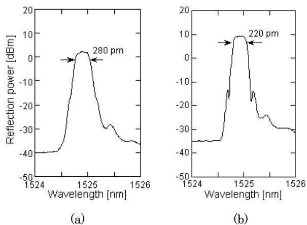
Figure 13 Reflection spectrum of FBG sensor at 1525 nm
