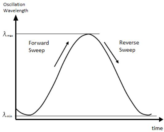
Figure 2 Lasing wavelength change of single-mode WSLS during wavelength sweeping
