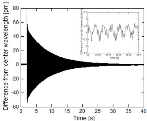
Figure 15 Result of vibration measurement at 1545 nm
