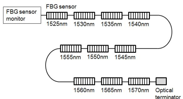
Figure 11 Measurement setup for reflection spectrum of FBG sensors
