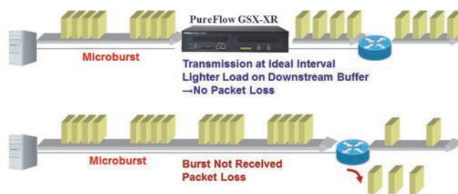
Figure 2 Packet Loss Caused by Microburst Traffic
