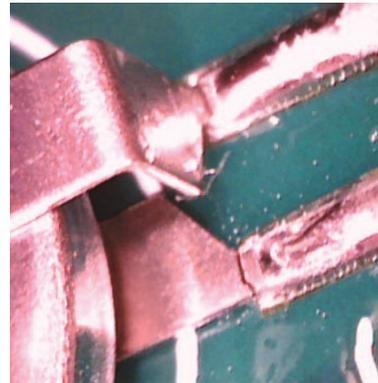
Figure 11 Fractured Backup Battery Lead
