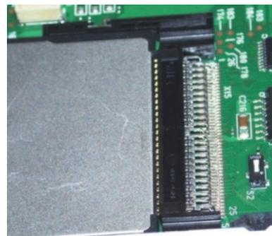
Figure 12 CF Card Slipping from Connector
