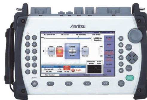
Figure 1 External View of MT9083 ACCESS Master
