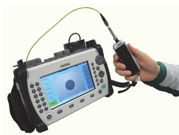
Figure 10 Example of G0306A Fiber Scope Use
