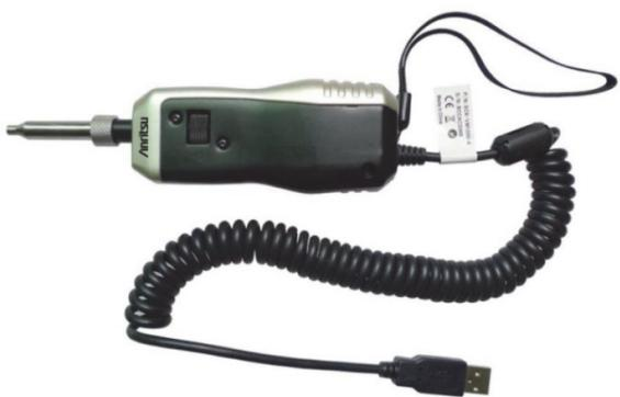
Figure 9 External View of G0306A FiberScope
