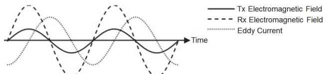
Figure 3 Relationship between Magnetic Field and Eddy Current
