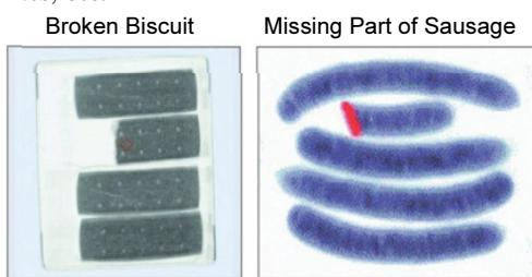
Figure 18 X-ray Image for Shape Detection
