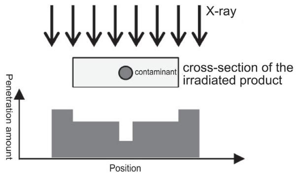
Figure 12 X-ray irradiation on a product with contaminant
