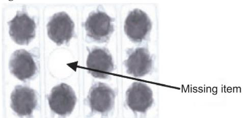
Figure 17 X-ray Image for Missing Product Detection
