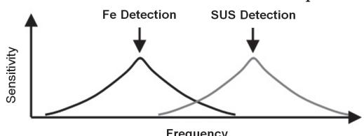
Figure 4 Relationship between Magnetic Field Frequency and Signal Levels
