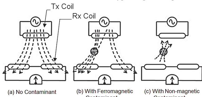
Figure 2 Principle of Metal Detector
