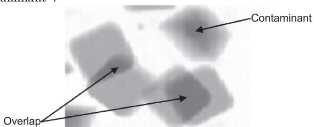
Figure 14 X-ray Image of Overlapping Products and Contaminant
