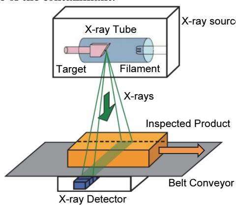
Figure 11 Principle of X-ray Inspection Systems
