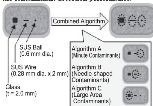
Figure 13 Concept of Combined Algorithm
