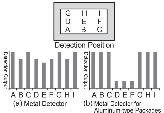
Figure 6 Relationship between Detection Sensitivity and Position
