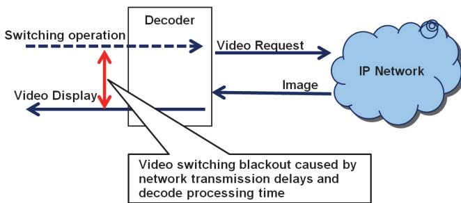
Figure 6 Cause of Video Switching Blackouts
