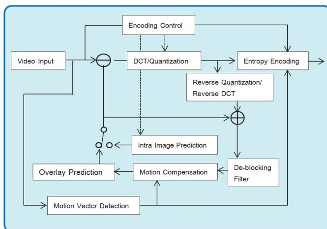
Figure 2 H.264 Encoder Circuit Diagram
