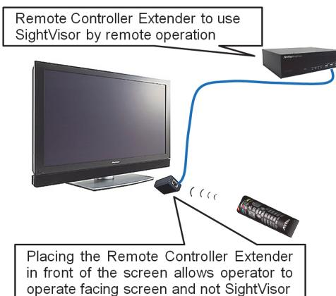
Figure 9 Remote Control Extender
