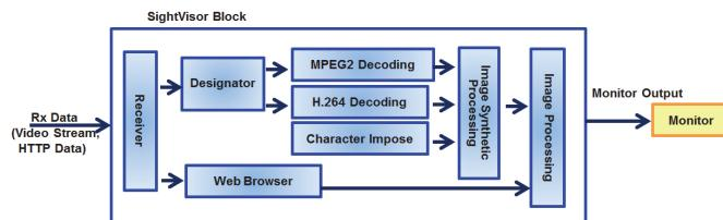
Figure 4 SightVisor Block Diagram
