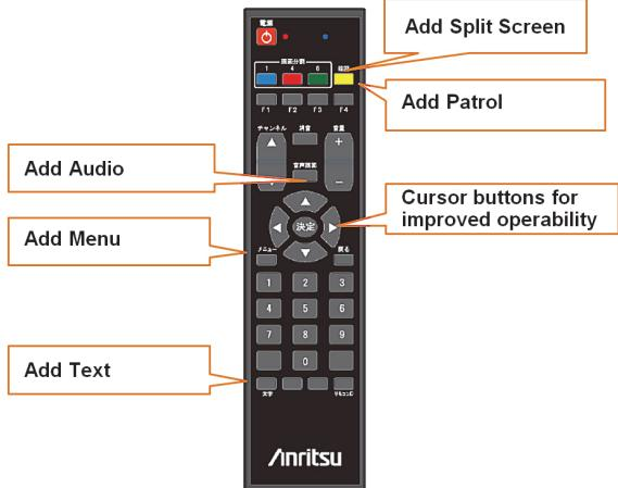
Figure 8 External View of Remote Control
