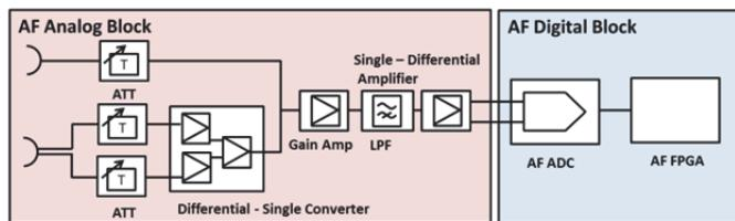
Figure 6 Audio Analyzer Block Diagram
