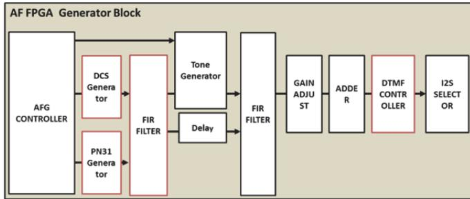
Figure 5 FPGA Signal Generator Block Diagram
