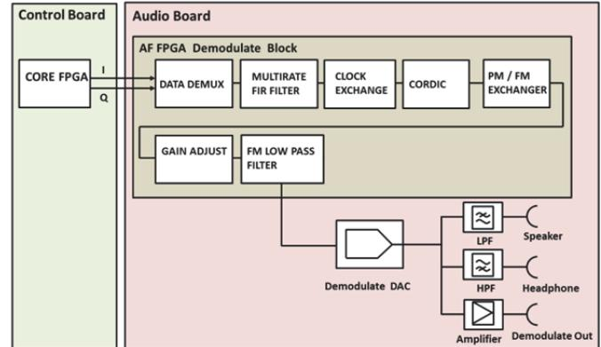
Figure 7 FM Demodulation Section
