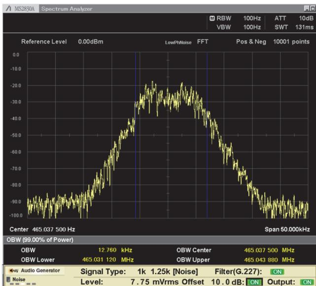
Figure 10 Occupied Frequency Bandwidth Measurement Screen
