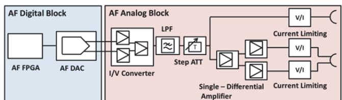
Figure 4 Audio Generator Block Diagram
