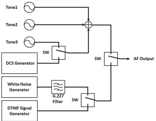
Figure 9 Audio Generator Concept Block Diagram
