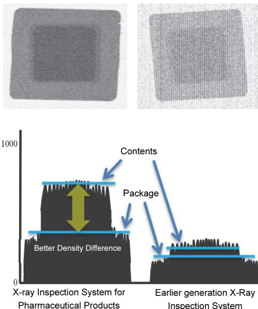
Figure 6 X-ray Penetration Picture and Density
