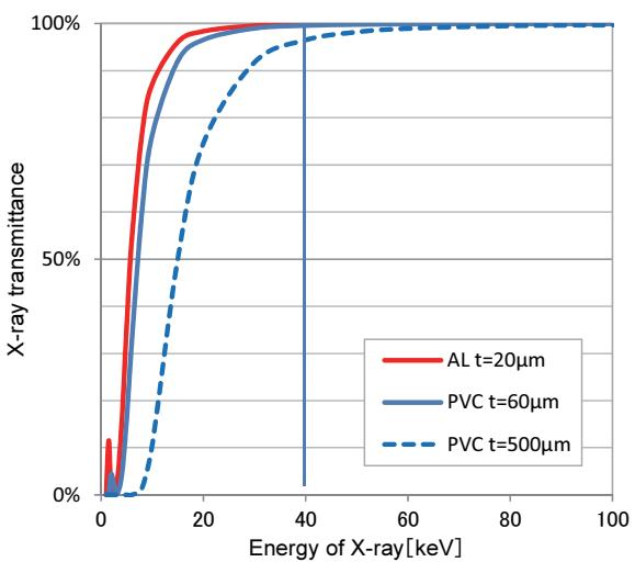
Figure 5 X-ray Transmittance
