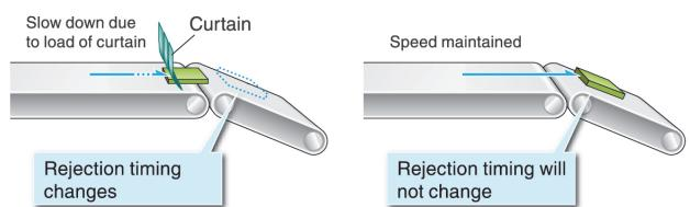
Figure 7 Effect of Protection Curtain
