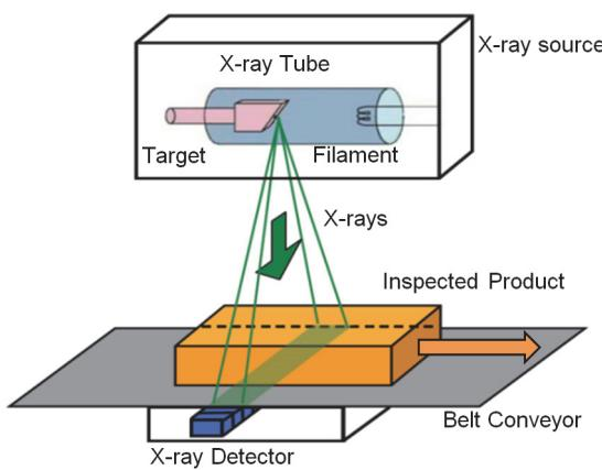
Figure 2 Principle of X-ray Inspection System
