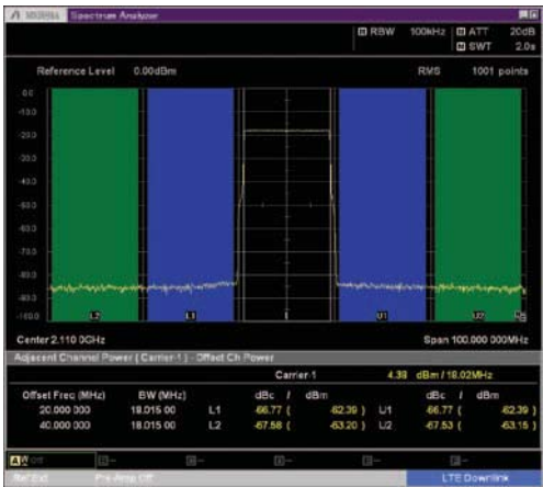
LTE FDD ACLR, 1 Carrier (E-TM1.1, Bandwidth 20 MHz)
