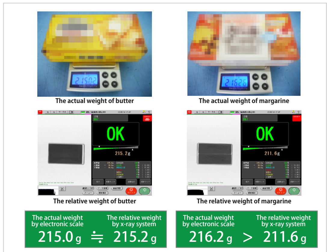
Fig. 3-1: Difference between the relative virtual weight and the actual weight
