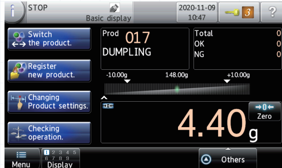
Fig.12 Zero point deviated at the plus side by a label
