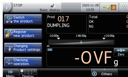
Fig.10 Zero set error by forgetting to attach a drive belt cover
