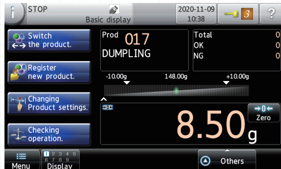
Fig.14 Zero point deviated at the plus side by rice grains
