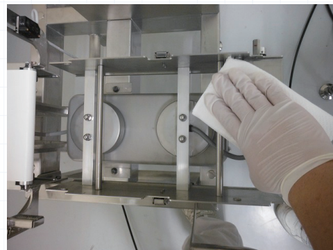
Fig.16 Remove a conveyor to clean a stand
