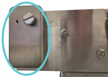
Fig.7 With a drive belt cover
