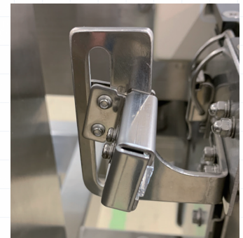
Fig.16: Reflection plate inclined to downward
