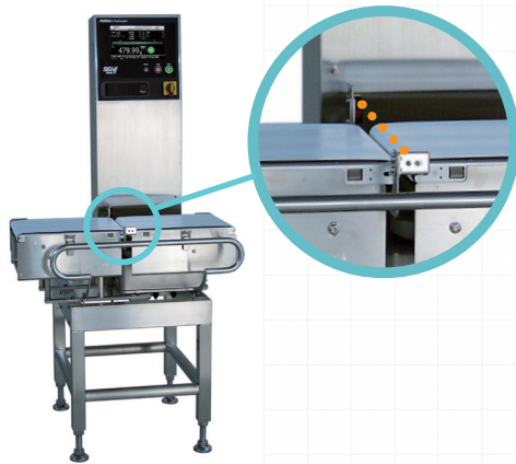
Fig.6: The position of the sensor for single unit model
