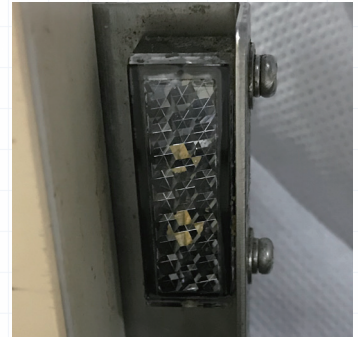
Fig.12: Dirt on the reflection plate
