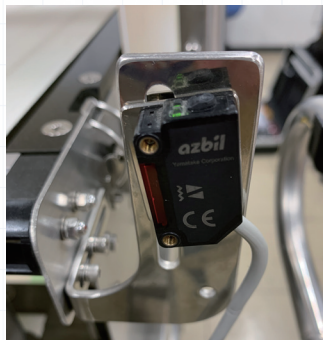
Fig.15: Photocell inclined to upward
