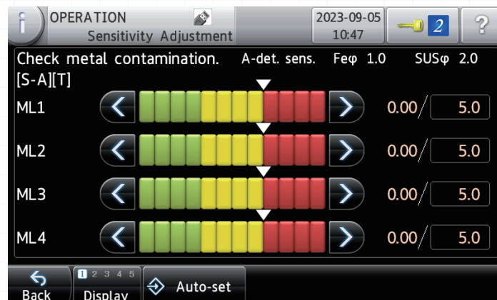
The indicator is fluctuating due to inverter noise
