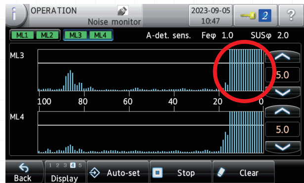
Result of changing the inverter frequency
