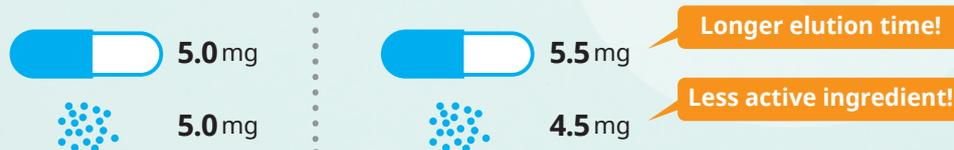
Because variability in the pre-filled (prelock) capsules results in **variability in the elution time and amount of active ingredient**, in addition to mass control of filled capsules, the mass of capsules prior to filling needs to be strictly controlled for highly active pharmaceutical preparations.
