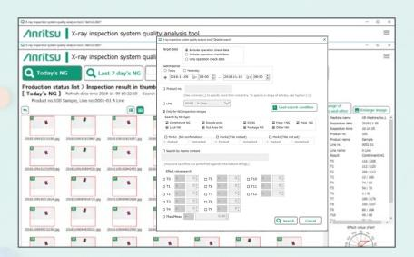
X-ray images are displayed in thumbnail view. If any foreign matter is detected, images of the NG product as well as of those before and after the product are displayed, making it possible to visually check for small foreign matter that the equipment cannot detect.
