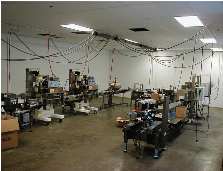
Wheelchair accessibility is essential on this line, so power is supplied to all of the machines from overhead, rather than through conduits on the floor.
