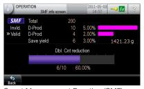
Smart Measurement Function (SMF) minimizes false rejects for products with inconsistent spacing.
