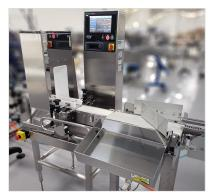
Example installation with dual flipper reject
