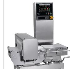
Metal detectors are also available as combos, paired with Anritsu SSV checkweighers.
