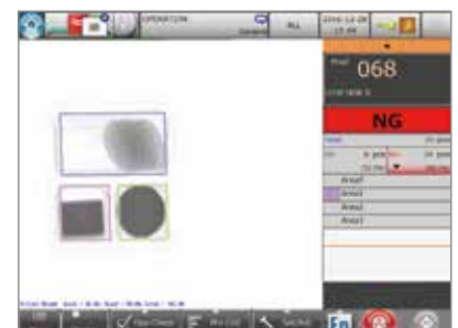
Insufficient amount of crackers
