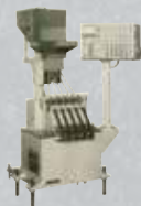
Checkweigher for Capsules K515 (1970)
