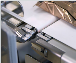
5mm-diameter conveyor roller for optimal product transfer of small products at high speeds
