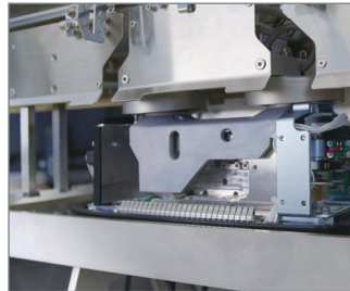
New digital force balance weigh cell with 2.5x higher resolution than previous model
