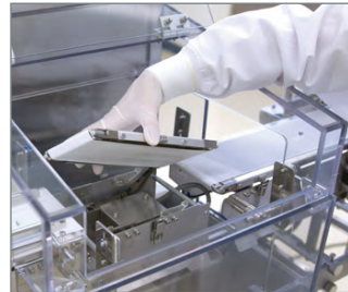
Easy tool-free conveyor/belt removal allows quick, simple cleaning and maintenance.
