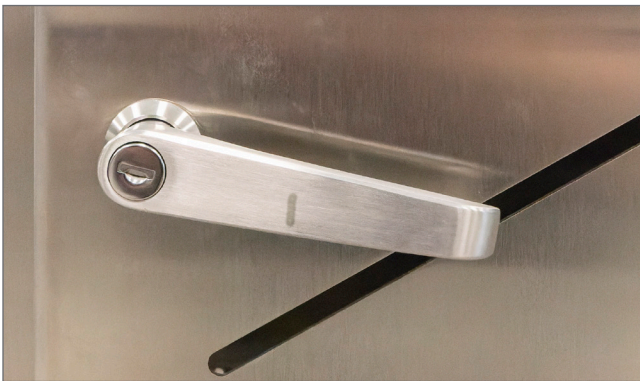
Locking door handle on reject bin
