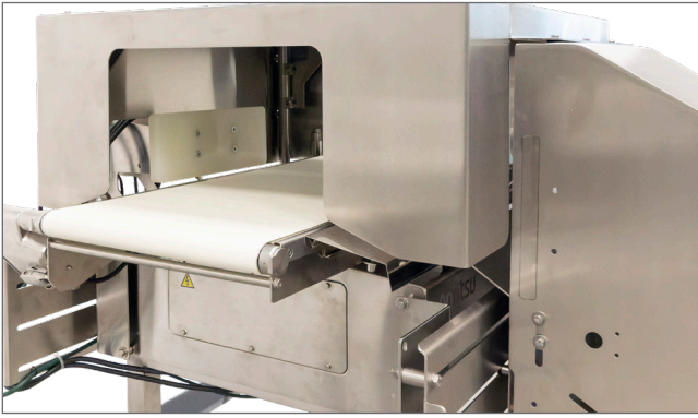
Pusher reject installed
