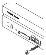
Figure 2.8-1 Removing the USB cap
