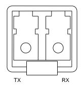
Figure A.5-1 10GBASE-LR module front view
