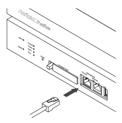
Figure 3.3.1-1 Connecting the console cable (device side)
