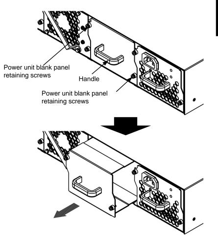
Figure 4.3.1-1 Removing the power unit blank panel
