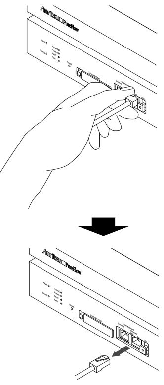
Figure 2.6.2-1 Removing the UTP cable
