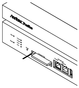
Figure 2.7-3 Removing the CF card
