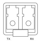
Figure A.7-1 1000BASE-LX module front view
