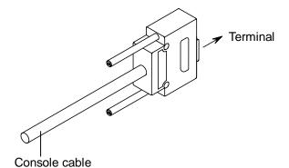
Figure 3.3.1-2 Connecting the console cable (terminal side)
