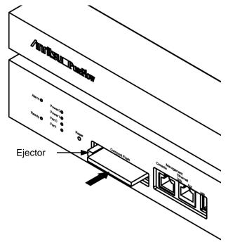
Figure 2.7-2 Inserting the CF card
