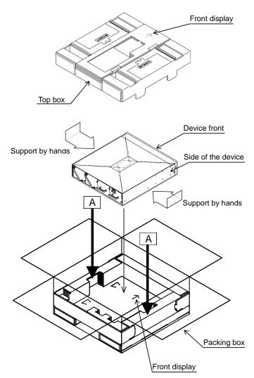
Figure 2.10.1-1 How to pack the NF7101C
