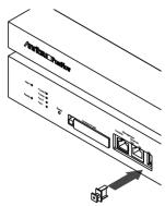
Figure 2.8-4 Attaching the USB cap
