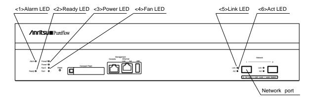
Figure 5.1-1 Names of LEDs
