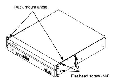
Figure 2.4.2-1 Attaching the rack mount angles
