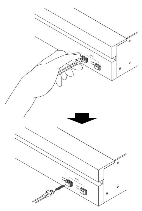
Figure 2.5.3.2-1 Removing the optical fiber cable
