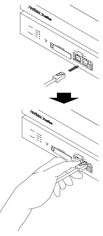
Figure 2.6.1-1 Inserting the UTP cable
