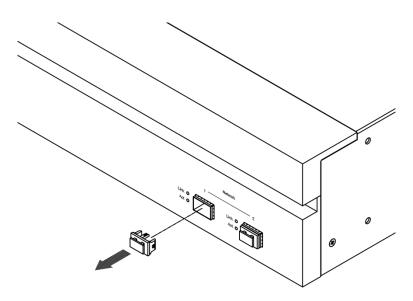
Figure 2.5.2.1-1 Removing the SFP cage plug
