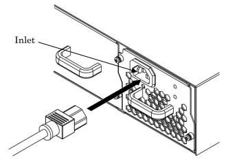
Figure 3.1-1 Connecting the AC power cord (inlet)
