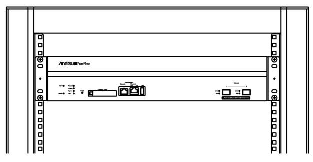
Figure 2.4.2-5 Mounting the NF7101C on the rack
