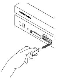
Figure 2.8-3 Removing the USB memory
