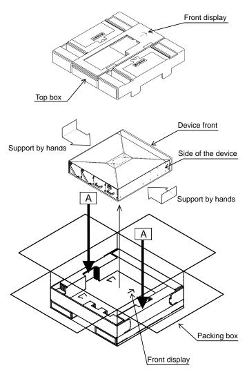
Figure 2.1.1-1 How to unpack the NF7101C
