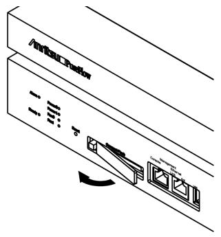
Figure 2.7-1 Removing the CF cap
