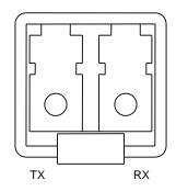
Figure A.6-1 1000BASE-SX module front view
