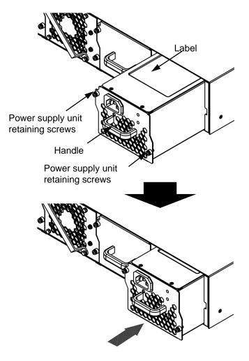
Figure 4.2.2-1 Attaching the power supply unit
