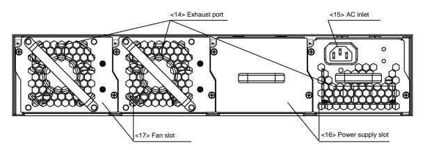
Figure 1.3-2 Rear view of device with part names
