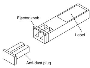
Figure 2.5-1 External view of SFP module (for LC connector)
