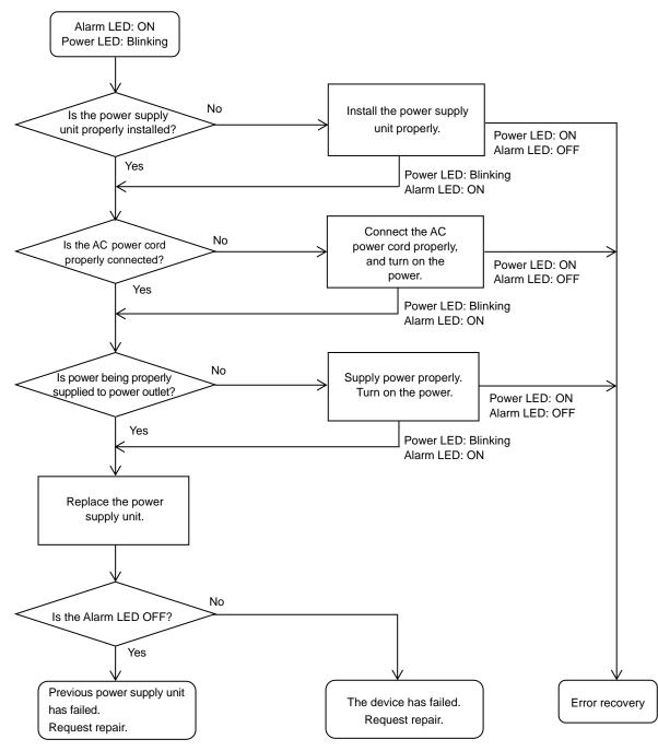
Figure 5.2.1-1 Error investigation flow when the Power LED is blinking
