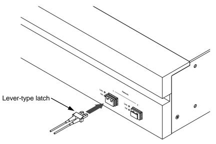
Figure 2.5.3.1-3 Connect the optical fiber cable
