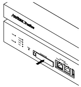
Figure 2.7-4 Attaching the CF cap
