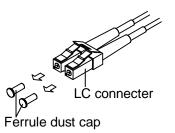
Figure 2.5.3.1-2 Removing the ferrule dust cap
