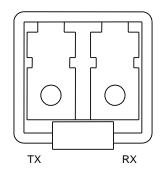
Figure A.4-1 10GBASE-SR module front view
