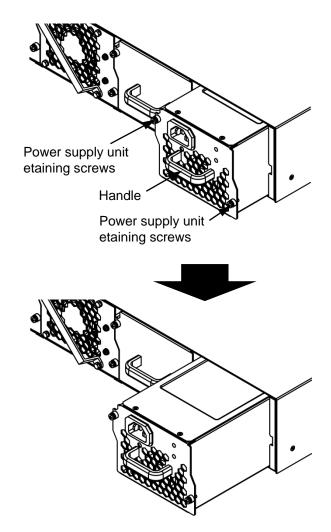
Figure 4.2.1-1 Removing the power supply unit
