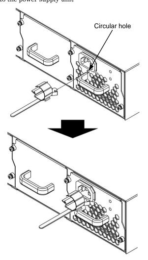
Figure 3.1-3 Clamping the AC power cord
