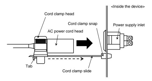
Figure 3.1-4 AC power cord clamp
