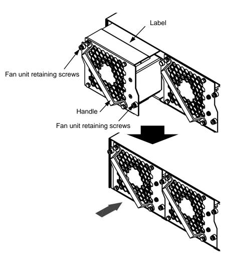
Figure 4.1.2-1 Attaching the fan unit
