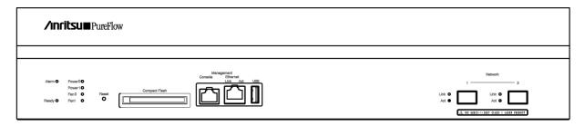
Figure 1.1-3 Front view of the NF7101C
