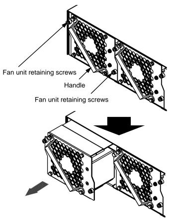
Figure 4.1.1-1 Removing the fan unit
