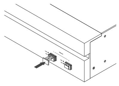
Figure 2.5.3.2-2 Attaching the dust-proof plug
