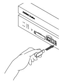
Figure 2.8-2 Connecting the USB memory
