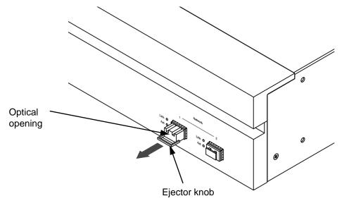
Figure 2.5.2.2-1 Removing SFP module
