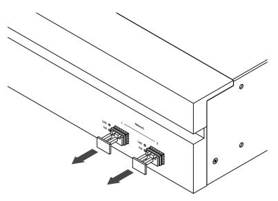
Figure 2.5.3.1-1 Removing the dust-proof plug
