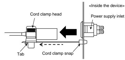
Figure 3.4-2 Unclamping the AC power cord
