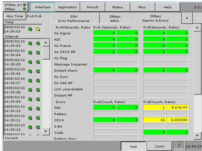
Figure 11 In-service analysis indicating problems in the investigated SDH network element.
