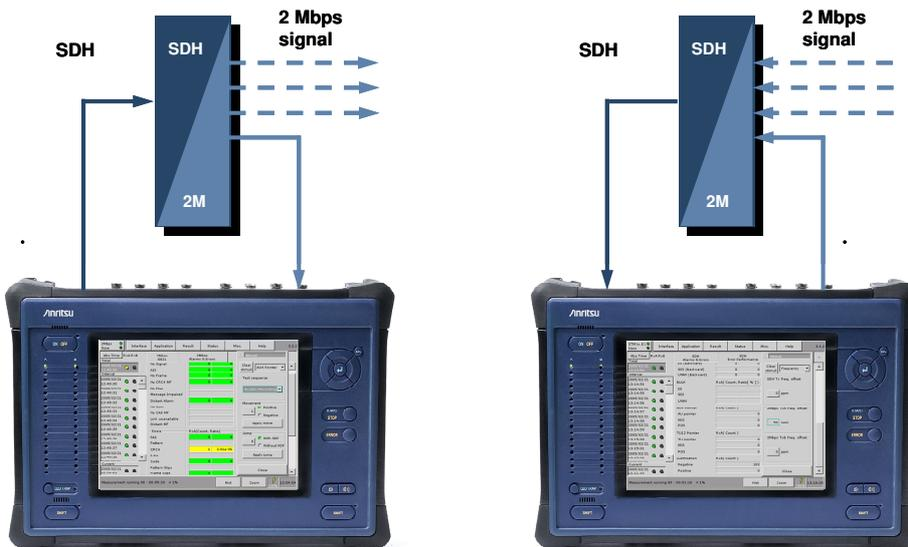
Figure 3 Out-of-service testing of SDH network elements.
