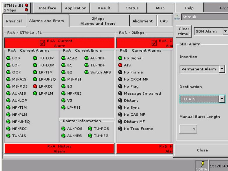
Figure 7 Check the SDH network element for correct handling of incoming maintenance signals.
