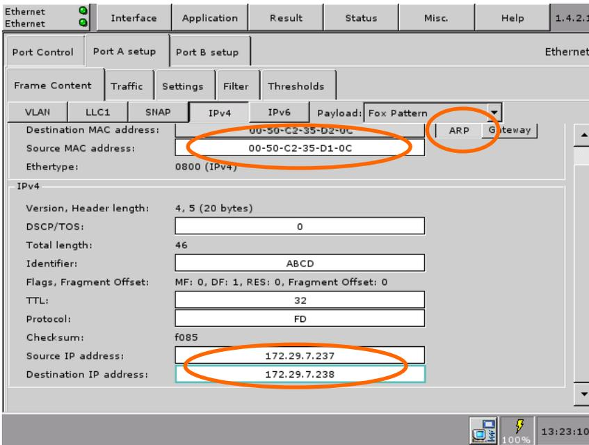
Figure 3 Setting of addresses for the Slave CMA 3000
