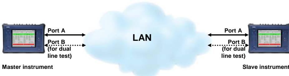
Figure 1 End-to-end RFC 2544 testing using two 3000's
