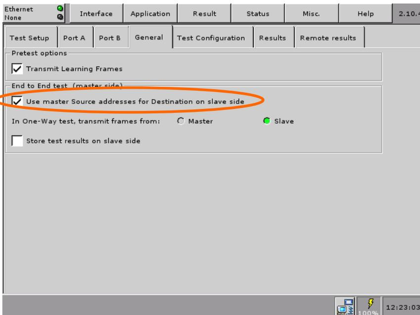
Figure 10 RFC 2544 General setup page of the Master CMA 3000
