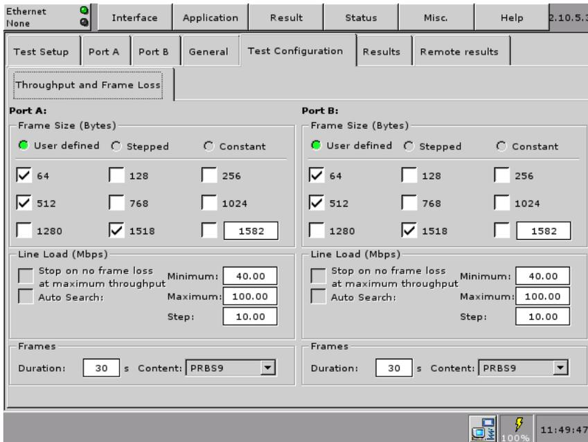
Figure 9 Detailed setup of Throughput test on the Master CMA 3000
