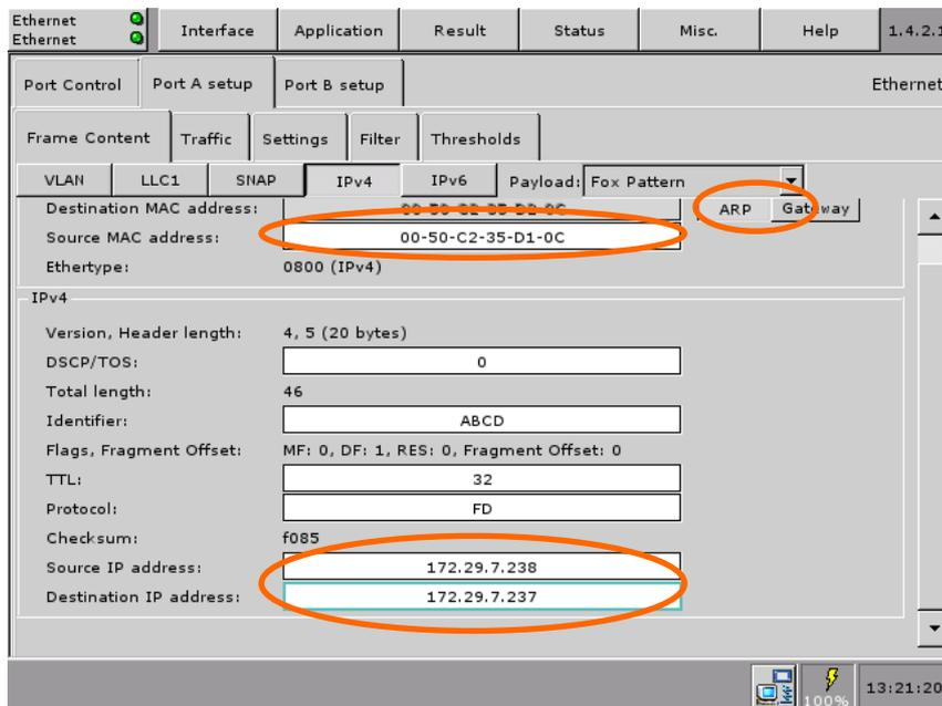
Figure 6 Setting of addresses for the Master CMA 3000
