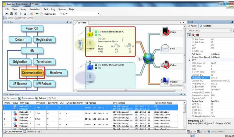
Figure 7. UE Connects to BTS1 (LTE)
