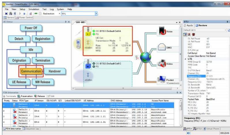
Figure 17. UE Connects to BTS1 (LTE)
