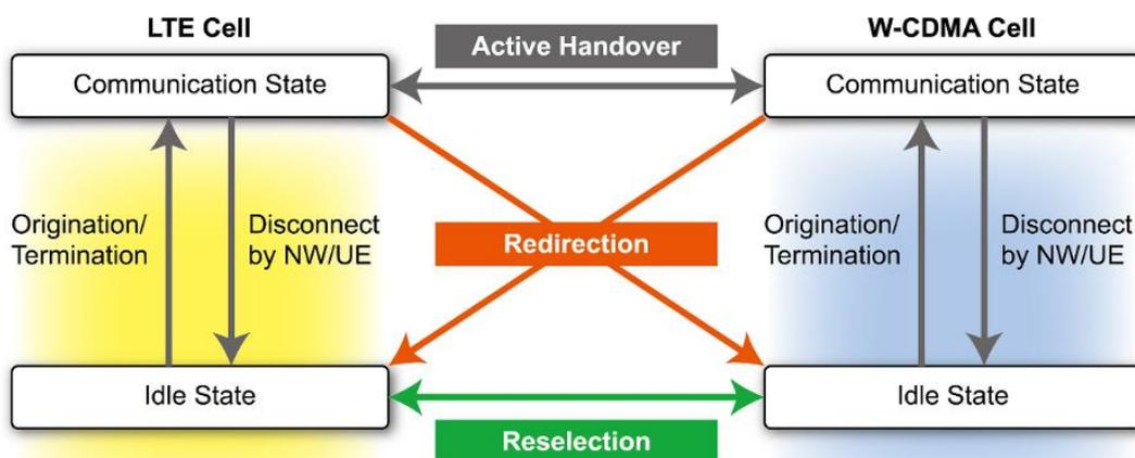
Figure 3. Case of UE Connection Cell in LTE and W-CDMA
