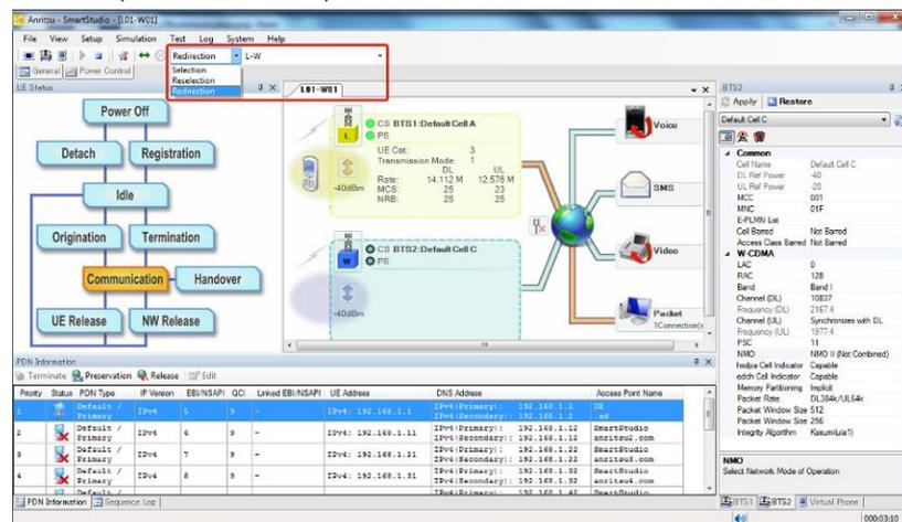
Figure 8. Set Redirection Test Mode
