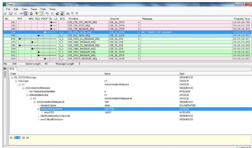
Figure 11. RRC Connection Release
