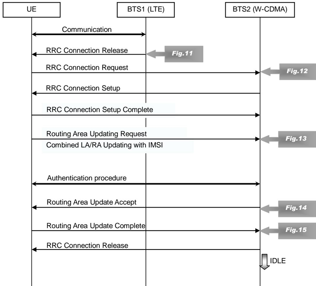
Figure 10. Protocol Sequence in LTE W-CDMA Rediection
