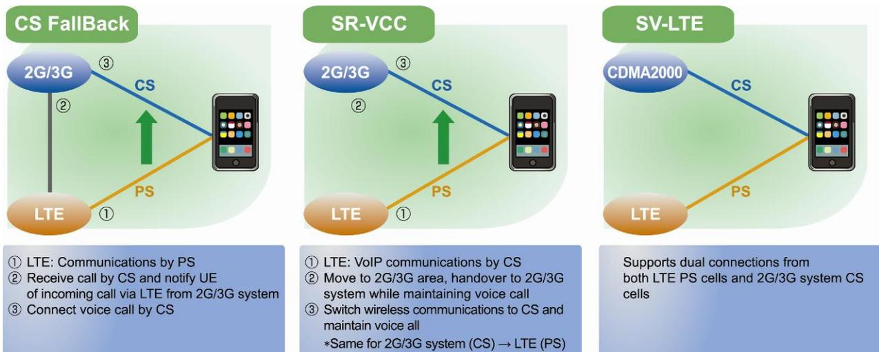
Figure 4. Technology Linked with 2G/3G System Circuit Switching
