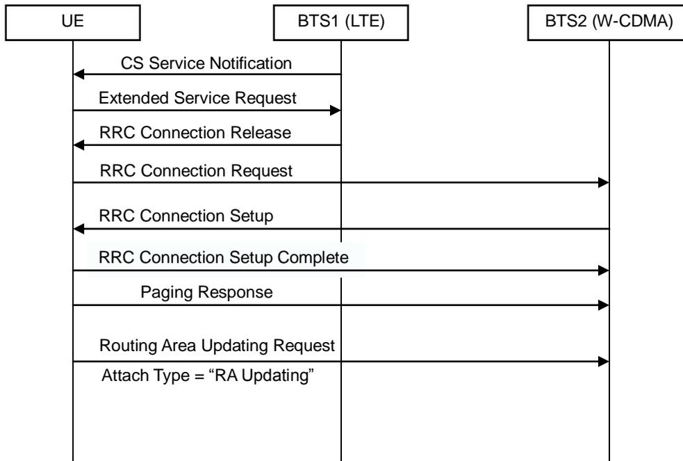
Figure 20. Protocol Sequence in LTE W-CDMA CS Fallback
