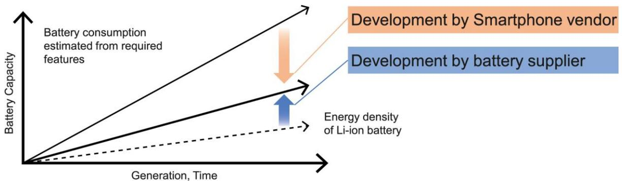
Figure 2. Gap between battery capacity required by smartphones and technical revolution in lithium battery technology
