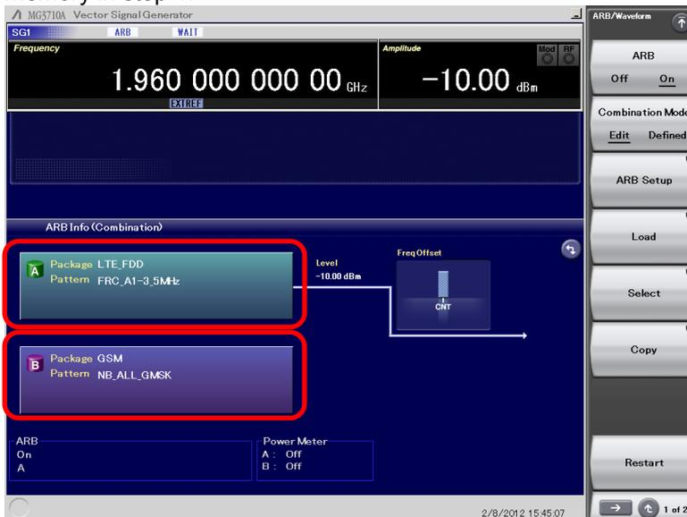
4. Set [Output A] and [Output B] shown in Mode at [ARB Setup] to output both waveform memories A and B.
