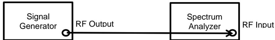
Figure 1. Measurement System
