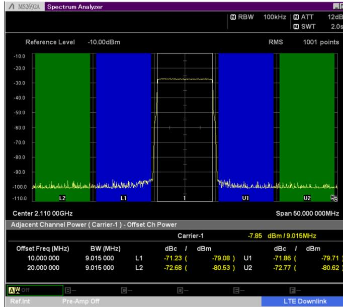
Fig. 4. ACLR (measured) for LTE FDD E-TM1.1 10MHz (Output Level: -7 dBm)
