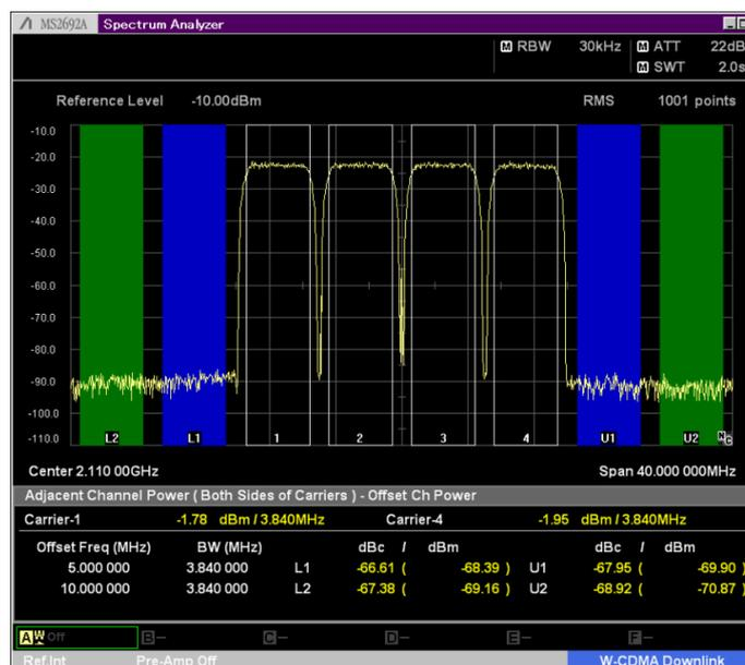
Fig. 3. ACLR (measured) for W-CDMA Test Model 1, 64DPCH x 4 Carrier (Output Level: + 5 dBm)
