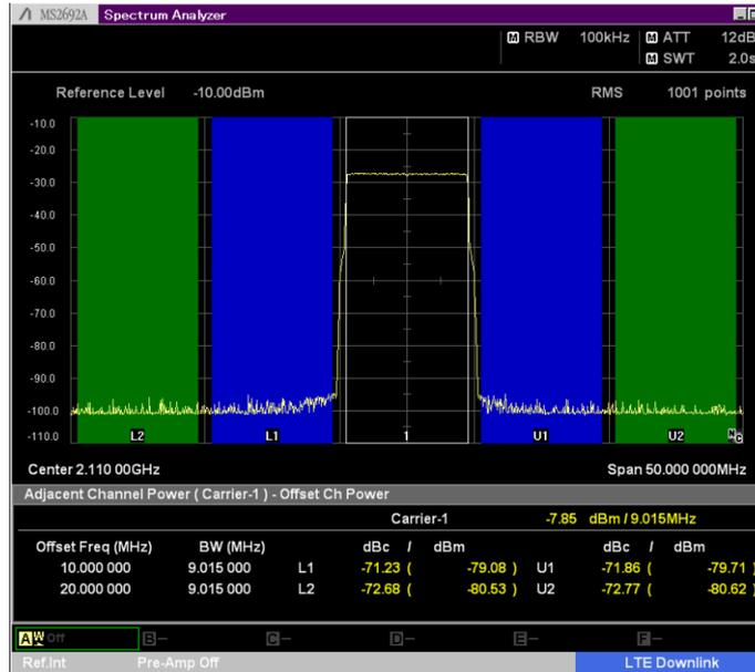
Fig. 4. ACLR (measured) for LTE FDD E-TM1.1 10MHz
