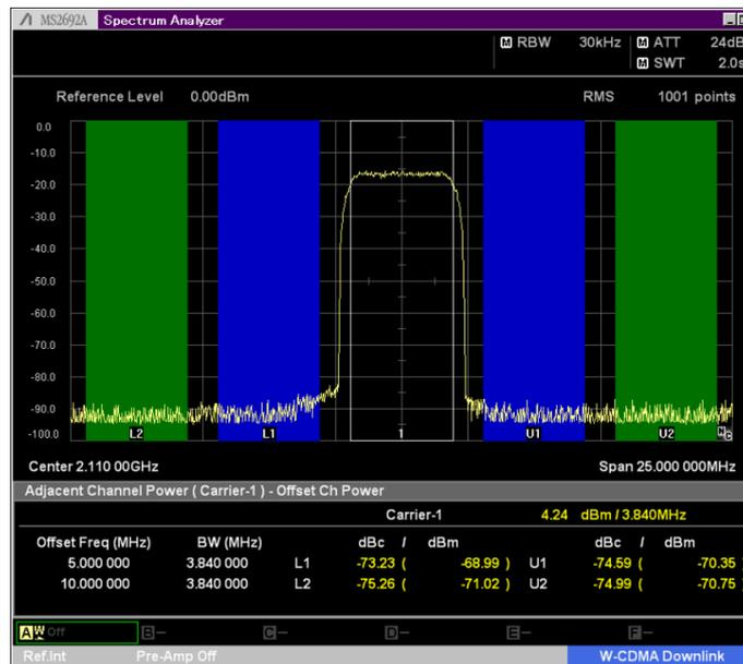
Fig 2. ACLR (measured) for W-CDMA Test Model 1, 64DPCH
