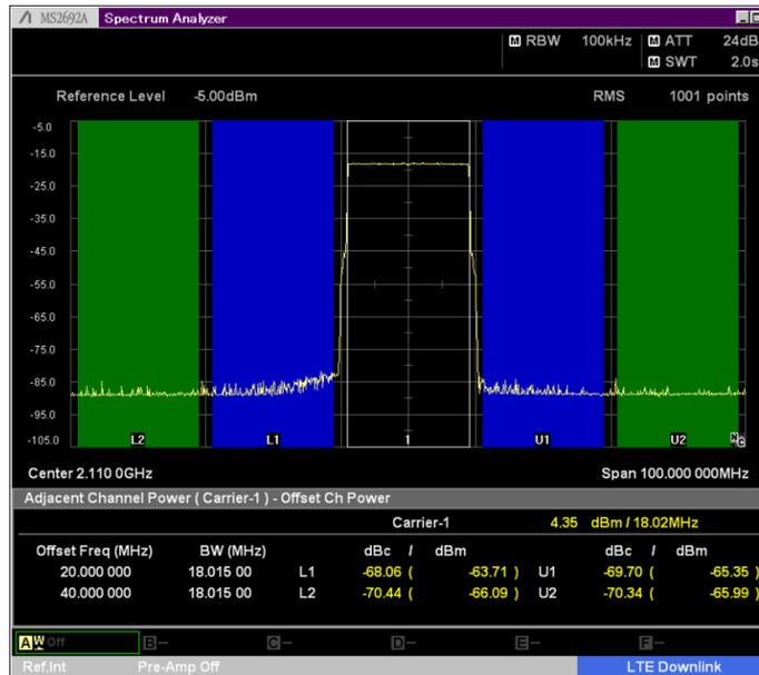
Fig. 5. ACLR (measured) for LTE FDD E-TM1.1 20 MHz
